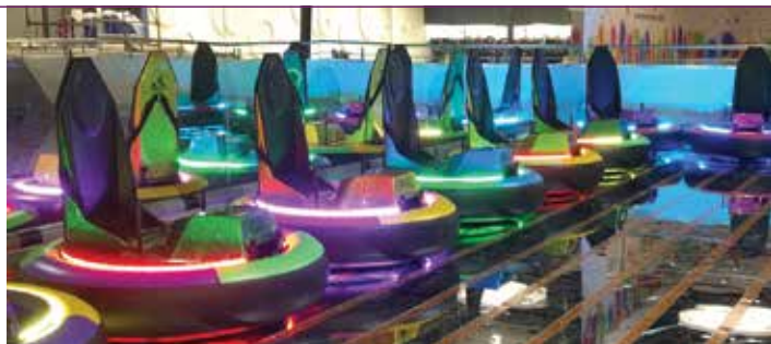
The Fun Company relies on the electrified floors that are part of bumper cars from RDC to run its cars nonstop.
